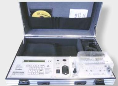
For testing of LSA arrester magazines equipped with GDT. The whole test equipment is fixed in a portable case with place for a lot of accessories (e.g. AC- adapter, test adapter for different kind of GDT magazines).
