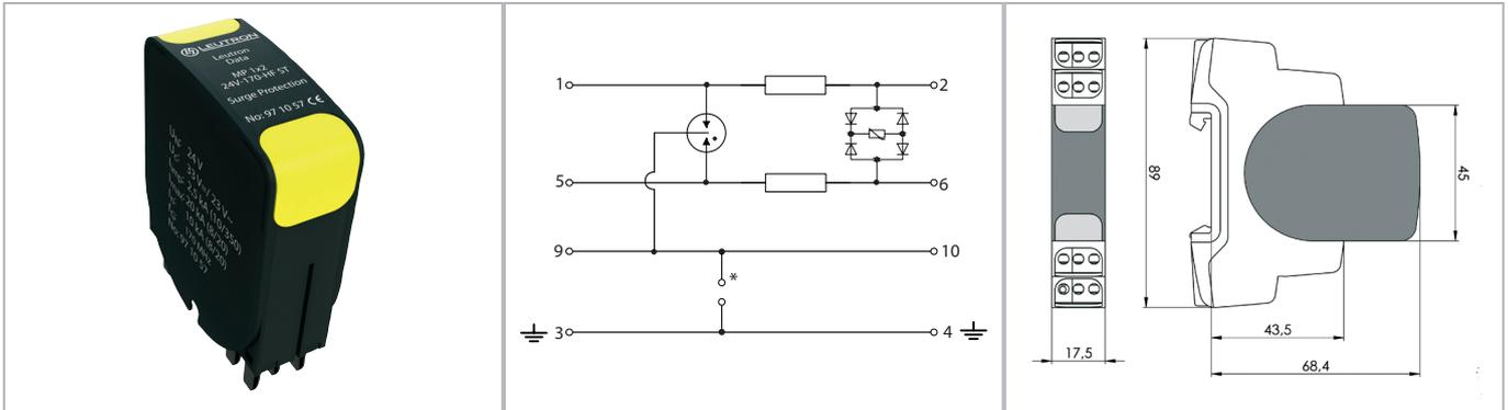
Fully pluggable two-parts arrester for signal lines for high frequency applications such as bus systems or video transmission. The protective module can be removed for test or maintenance purposes without changing the line impedance and therefore influencing the signal level. The base part can remain in the installation without manipulating or removing any wire.
