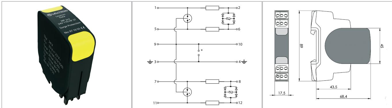
**Fully pluggable two-parts arrester for signal lines for high frequency applications such as bus systems or video transmission. The protective module can be removed for test or maintenance purposes without changing the line impedance and therefore influencing the signal level. The base part can remain in the instalation without manipulating or removing any wire.**
