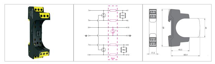
Indirect earthing of the signal shielding: The MP Base 2x2-R GDT HF has a gas discharge tube linked between the shield connectors 9/10 (GND) and the DIN rail and earth connector. Therefore a galvanic insulation between the signal shield and the earth connection (PE) can be reached. For accepting a MP module.
