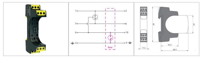
Indirect earthing of the signal shielding: The MP Base 1x2 GDT has a gas discharge tube linked between the shield connectors 9/10 (GND) and the DIN rail and earth connector. Therefore a galvanic insulation between the signal shield and the earth connection (PE) can be reached. For accepting a MP module.
