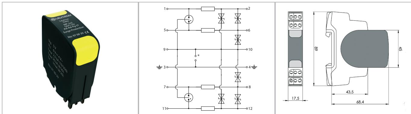
**Fully pluggable two-parts arrester for signal lines. The protective module can be removed for test or maintenance purposes without changing the line impedance and therefore influencing the signal level. The base part can remain in the instalation without manipulating or removing any wire.**
