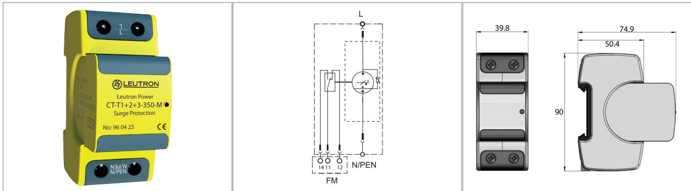
**Combined arrester with rare-gas-filled spark gap and very low protection level < 1.0 kV for the use between L - N wire. They provide extremely high discharge capacity with at the same time very low protection levels and they also do not need any damageable internal or external electronic trigger.**
