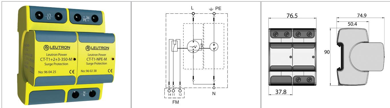
**Combined arrester with rare-gas-filled spark gap and very low protection level < 1.0 kV for the use in single-phase TT and TN systems. They provide extremely high discharge capacity with at the same time very low protection levels and they also do not need any damageable internal or external electronic trigger.**
