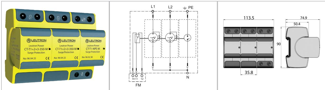
**Combined arrester with rare-gas-filled spark gap and very low protection level < 1.0 kV.** They provide extremely high discharge capacity with at the same time very low protection levels and they also do not need any damageable internal or external electronic trigger.
