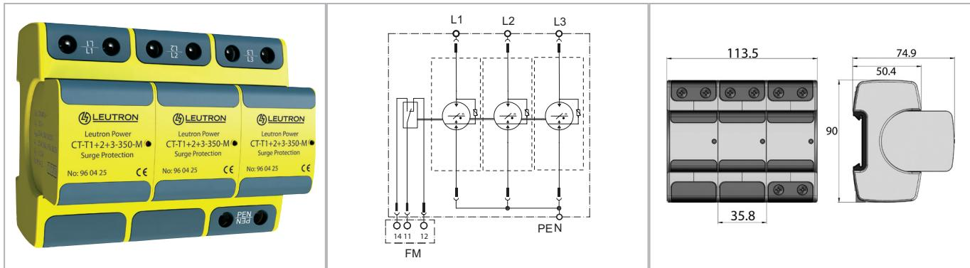
**Combined arrester with rare-gas-filled spark gap and very low protection level < 1.0 kV for the use in three-phase TNC systems. They provide extremely high discharge capacity with at the same time very low protection levels and they also do not need any damageable internal or external electronic trigger.**
