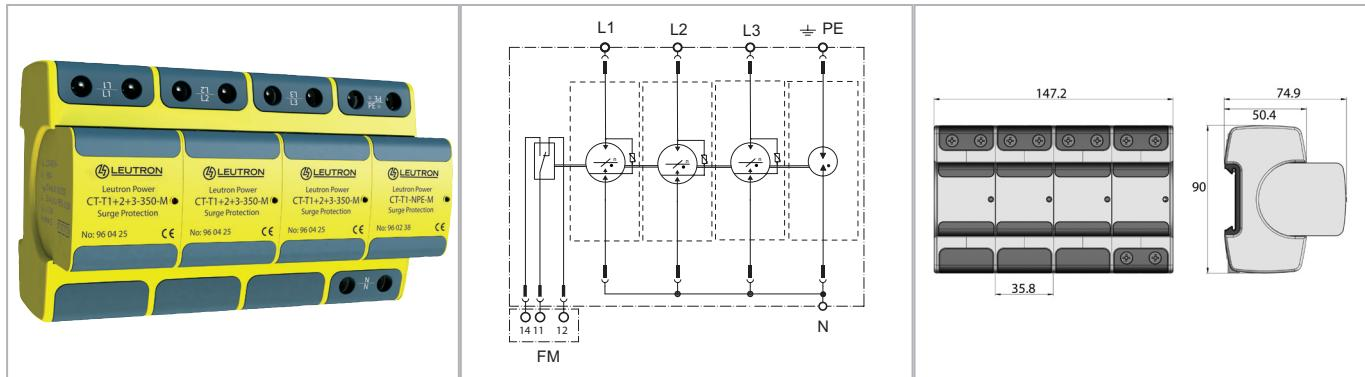
**Combined surge arrester with rare-gas-filled spark gap and very low protection level < 1.0 kV for the use in three-phase TT and TN-S systems. They provide extremely high discharge capacity with at the same time very low protection levels and they also do not need any damageable internal or external electronic trigger.**
