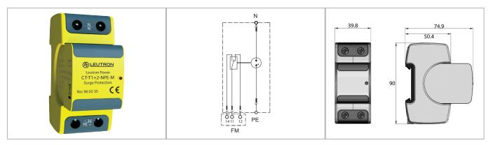
Lightning current cappable and rare-gas-filled summation current spark gap for the use between N - PE wire. They provide extremely high discharge capacity with at the same time very low protection levels and they also do not need any damageable internal or external electronic trigger.
