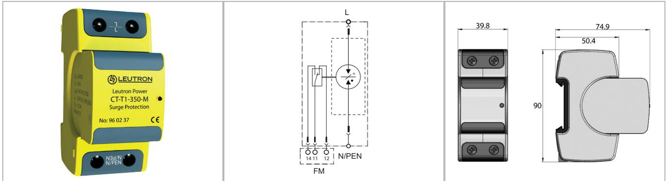
**Lightning current discharge arrester (class I) with rare-gas-filled spark gap for the use between L - N wire. They provide extremely high discharge capacity with at the same time very low protection levels and they also do not need any damageable internal or external electronic trigger.**
