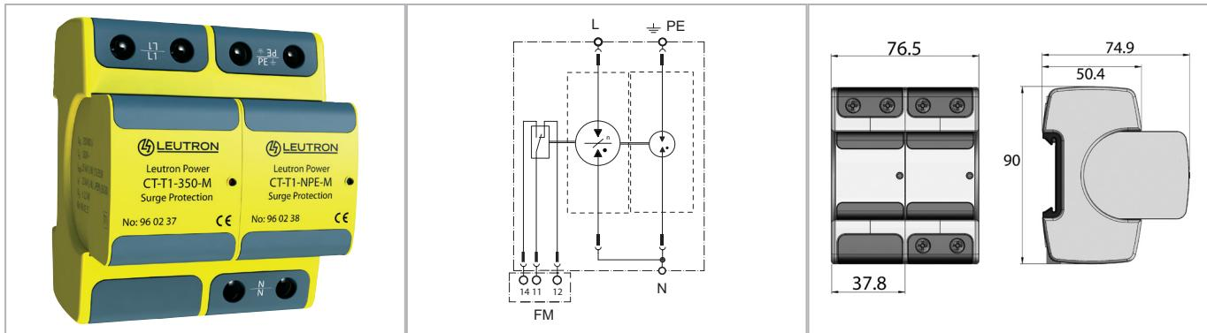
**Lightning current discharge arrester (class I) with rare-gas-filled spark gap for the use in single-phase TT and TN systems. They provide extremely high discharge capacity with at the same time very low protection levels and they also do not need any damageable internal or external electronic trigger.**
