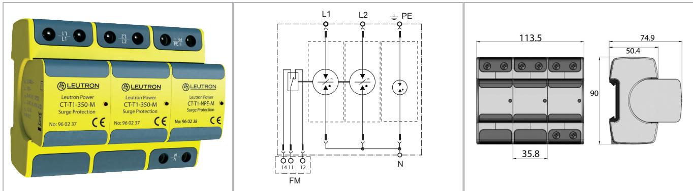
Multi-pole lightning current arrester (class I) for 2-phase TT systems. They provide extremely high discharge capacity with at the same time very low protection levels and they also do not need any damageable internal or external electronic trigger.
