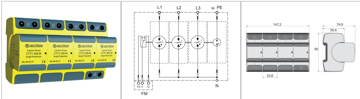
**Lightning current discharge arrester (class I) with rare-gas-filled spark gap for the use in three-phase TT and TN-S systems. They provide extremely high discharge capacity with at the same time very low protection levels and they also do not need any damageable internal or external electronic trigger.**
