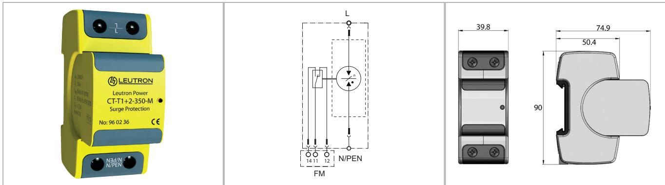
**Lightning current discharge arrester with rare-gas-filled spark gap and very low protection level < 1.5 kV for the use between L - N wire. They provide extremely high discharge capacity with at the same time very low protection levels and they also do not need any damageable internal or external electronic trigger.**
