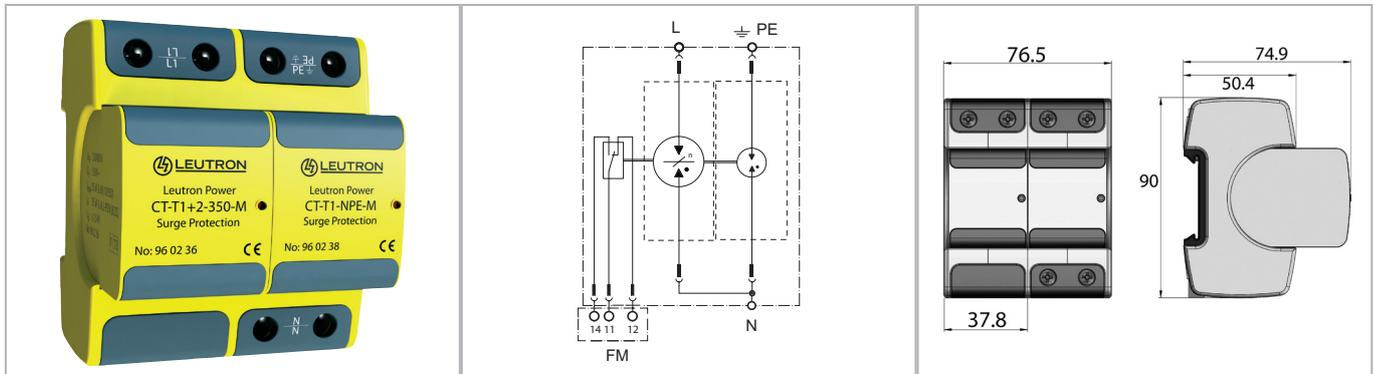
**Lightning current discharge arrester with rare-gas-filled spark gap and very low protection level < 1.5 kV for the use in single-phase TT and TN systems. They provide extremely high discharge capacity with at the same time very low protection levels and they also do not need any damageable internal or external electronic trigger.**
