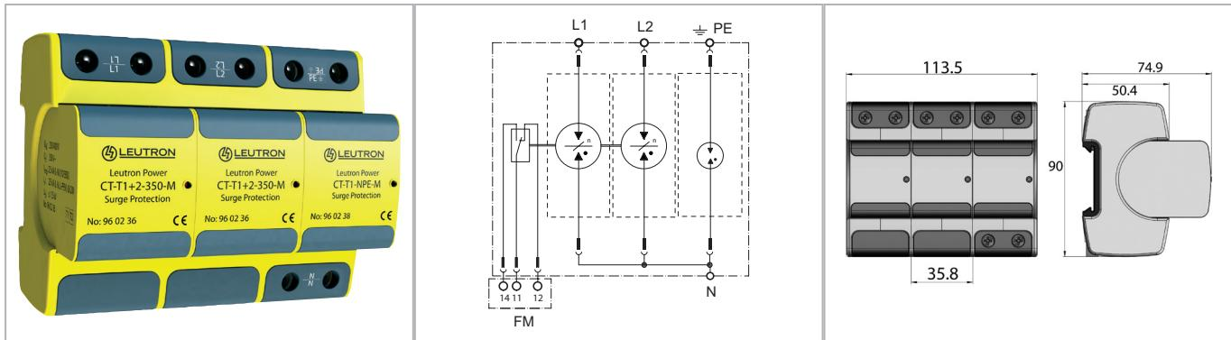
**Lightning current discharge arrester with rare-gas-filled spark gap and very low protection level < 1.5 kV for the use in 2-phase TT systems. They provide extremely high discharge capacity with at the same time very low protection levels and they also do not need any damageable internal or external electronic trigger.**
