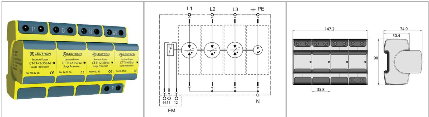
**Lightning current discharge arrester with rare-gas-filled spark gap and very low protection level < 1.5 kV for the use in three-phase TT and TN-S systems. They provide extremely high discharge capacity with at the same time very low protection levels and they also do not need any damageable internal or external electronic trigger.**
