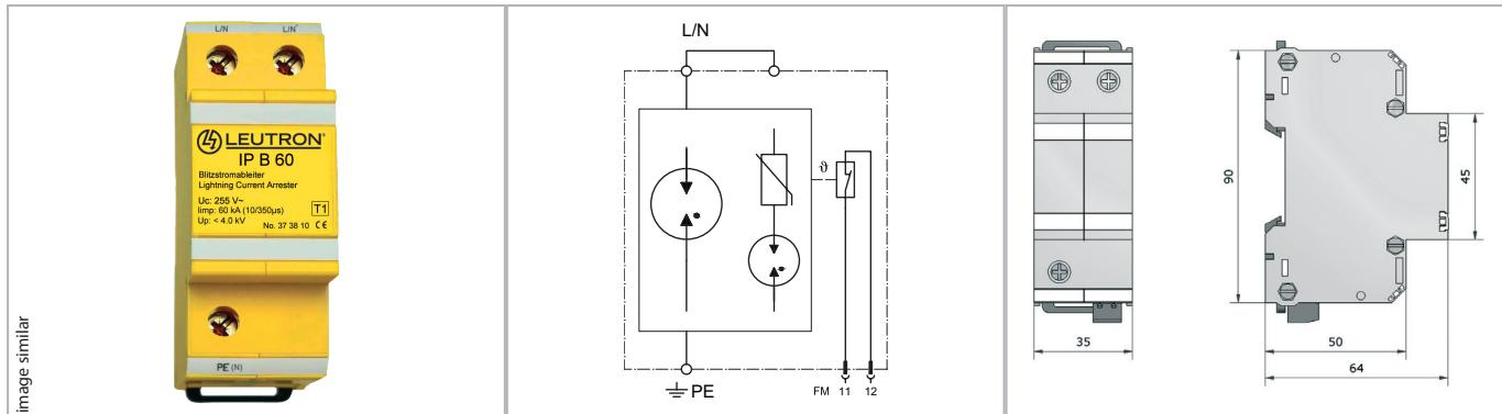
**Single pole SPD for use as equipotential bonding lightning surge protection in different kind of power net systems. Lightning current discharge arrester (class I) with rare-gas-filled spark gap for the use in single-phase TT and TN systems. Applicable at the boundaries LPZ 0A - 1 and higher.**
