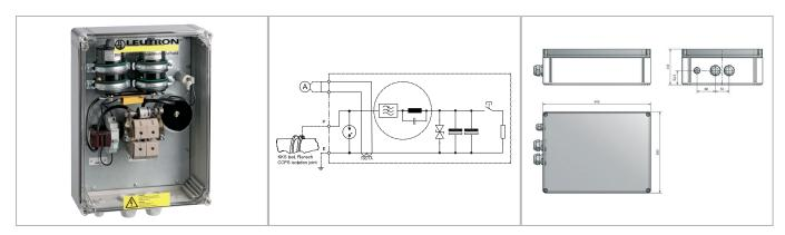
With an active cathodic corrosion protection the installation is permanently protected against the electrochemical process of corrosion. For that matter a grid supplied rectifier is inserted between the installation (e.g. a pipeline) and an anode that serves as earth electrode. By connecting two or three PLPro units in parallel the overall current can be elevated up to 80 respectively 120 A.
