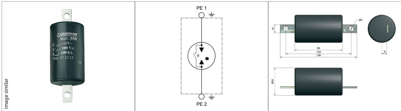
A rare-gas-filled spark gap for the lightning protection equipotential bonding, the insulation of electrically separated parts and the bridging of insulating flanges of gas pipelines. Weather-resistant, moulded metal/ceramic isolating spark gap with terminal lugs for M8 screw connection. Waterproof moulded in polyurethan diecast. Protection of power supply of dc
