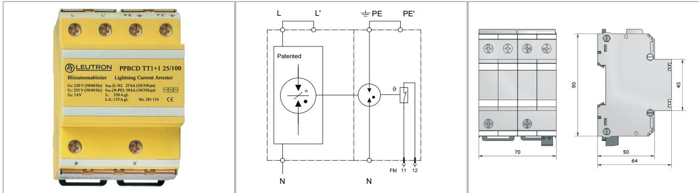
**Combined multi-pole arrester for 1-phase TT systems. Two-pole combined arrester for the protection of low-voltage consumers' installations in industry, business and residential areas against transient surges caused by lightning (LEMP) or switching actions in the network (SEMP).**
