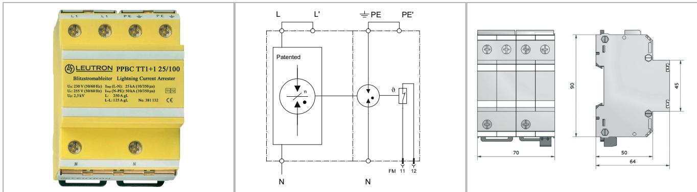
**Two-pole combined arrester for the protection of low-voltage consumers' installations in industry, business and residential areas against transient surges caused by lightning (LEMP) or switching actions in the network (SEMP). Combined multi-pole arrester for 1-phase TT systems.**
