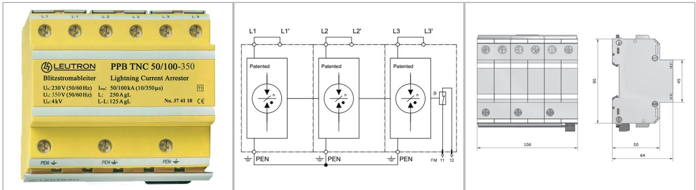
**Lightning current discharge arrester (class I) with rare-gas-filled spark gap for the use in three-phase TNC systems. Applicable at the boundaries LPZ OA - 1 and higher**
