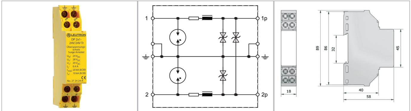
EMC filter for data and signal lines combined with surge protection enables smooth operation of sensitive electronic equipment in rough environment.
