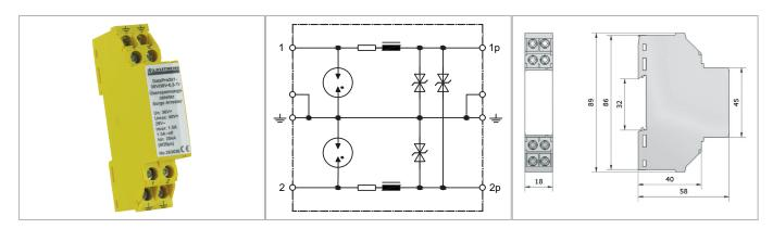
EMC filter for data and signal lines combined with surge protection enables smooth operation of sensitive electronic equipment in rough environment. Lightning current and surge voltage protection for particularly long signal and bus lines. Thanks to the extremely low volume resistance (impedance only  $0.3\Omega$ ) no noteworthy signal losses occur. It is a combined arrester to protect two single wires.
