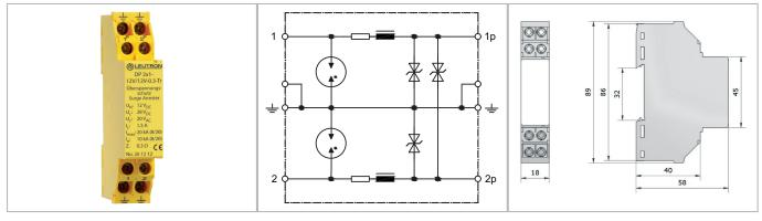
EMC filter for data and signal lines combined with surge protection enables smooth operation of sensitive electronic equipment in rough environment. Lightning current and surge voltage protection for particularly long signal and bus lines. Thanks to the extremely low volume resistance (impedance only  $0.3\Omega$ ) no noteworthy signal losses occur. It is a combined arrester to protect two single wires.
