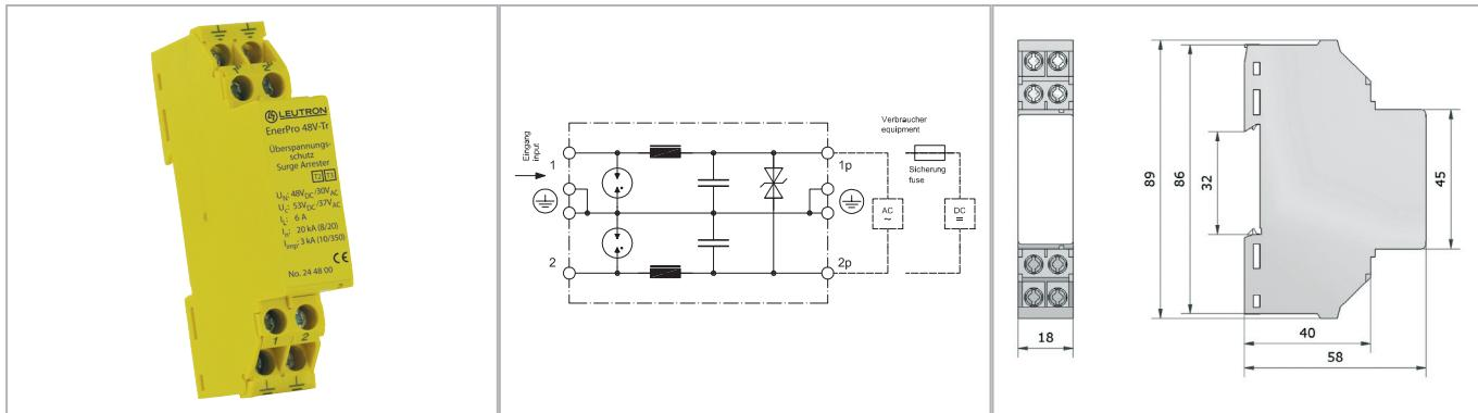
**Two-pole SPD type 2+3 (class II+III) with gas discharge tubes (GDT) and suppressor diodes for operating currents up to 6 A.**
