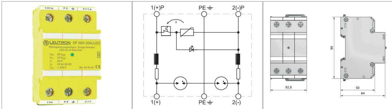
**Two-pole SPD for operating current up to 20 A in looped-in wiring, with disconnection device without interruption of the power supply.**
