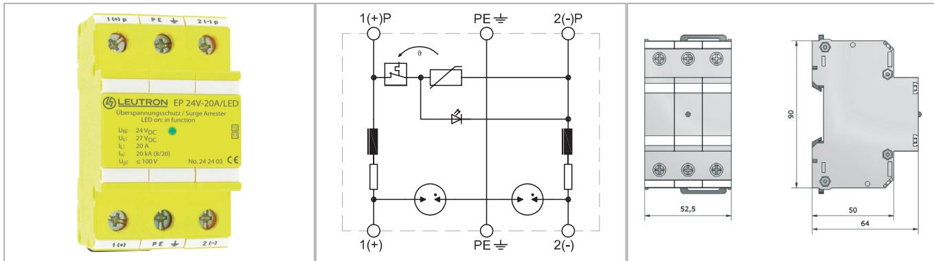
**Two-pole SPD for operating current up to 20 A in looped-in wiring, with disconnection device without interruption of the power supply. A very low protection level allows the use as SPD Typ 3 (class III).**
