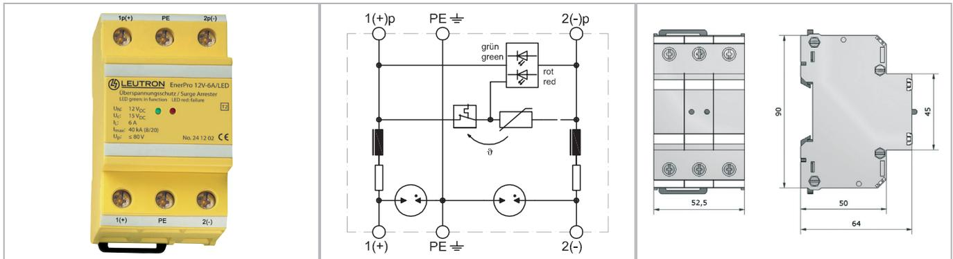
**Surge voltage arrester for electrical and electronic devices in looped-in wiring, with disconnection device without interruption of the power supply. A very low protection level allows the use as SPD Typ 3 (class III).**
