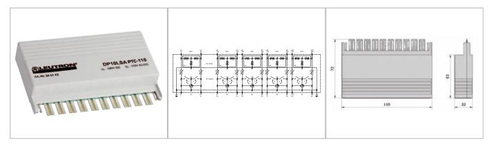
Surge voltage arrester with surge current protection via PTC thermistors. Designed for telecommunication lines as a pluggable module with 10 pair of wires (DA) for LSA (IDC) disconnection modules.
