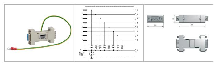
Surge voltage arrester for serial interfaces RS232/RS422/RS485. The multi pole surge protective plug adapter make serial interfaces of computers or controll systems secure of transient overvoltages.
