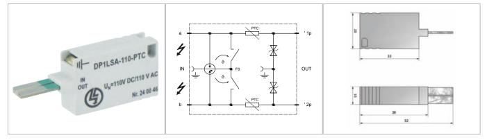
Surge protection device for data and signal lines in measuring systems and automatic control devices. Surge voltage protection connector for 1 DA, with surge current protection via PTC thermistors and fail-safe contact for LSA (IDC) disconnection modules.
