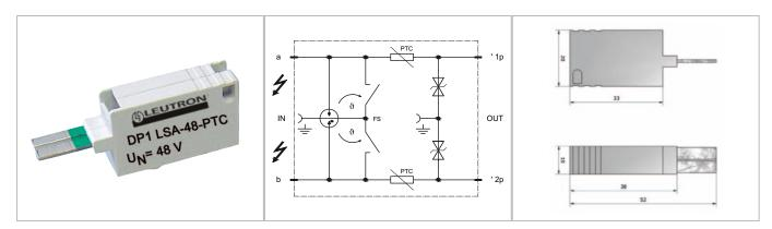
Surge protection device for data and signal lines in measuring systems and automatic control devices. Surge voltage protection connector for 1 DA, with surge current protection via PTC thermistors and fail-safe contact for LSA (IDC) disconnection modules.
