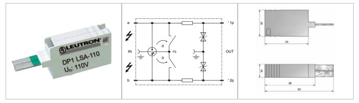
Surge voltage protective module for one pair of wires for measuring and control systems, in LSA (IDC) disconnection modules. The protective module provides coarse and fine protection in LSA systems (construction form 2). Surge voltage protection connector for 1DA, with fail-safe contact.
