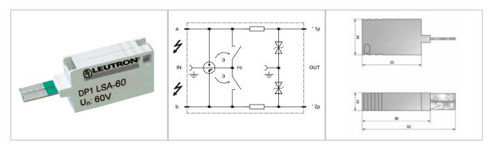
Surge voltage protective module for one pair of wires for measuring and control systems, in LSA (IDC) disconnection modules. The protective module provides coarse and fine protection in LSA systems (construction form 2). Surge voltage protection connector for 1DA, with fail-safe contact.
