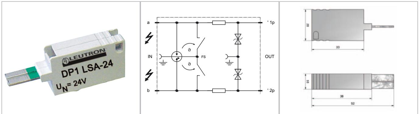
Surge voltage protective module for one pair of wires for measuring and control systems, in LSA (IDC) disconnection modules. The protective module provides coarse and fine protection in LSA systems (construction form 2). Surge voltage protection connector for 1DA, with fail-safe contact.
