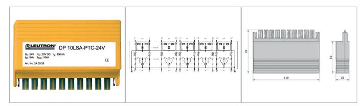
Surge voltage arrester with surge current protection via PTC thermistors. Designed for telecommunication lines as a pluggable module with 10 pair of wires (DA) for LSA (IDC) disconnection modules.
