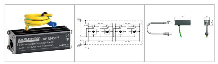
Compact surge protective module for the protection of data networks, and network devices such as hubs, switches, server. The adaptor plug style provides an easy application in cable ducts or directly at the terminal equipment. All 8 signal lines (4 pair of wires) are protected simultaneously.
