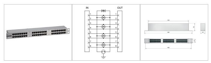
Compact surge protective module in 19" housing with only 1 HE (45 mm) for the protection of data networks and network devices such as hubs, switches, server and desktop computer. Easy installation and wiring in all 19" distribution and server racks possible. •All 8 signal lines (4 pair of wires) are protected simultaneously.
