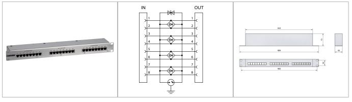
Compact surge protective module in 19" housing with only 1 HE (45 mm) for the protection of data networks and network devices such as hubs, switches, server and desktop computer. Easy installation and wiring in all 19" distribution and server racks possible. All 8 signal lines (4 pair of wires) are protected simultaneously.
