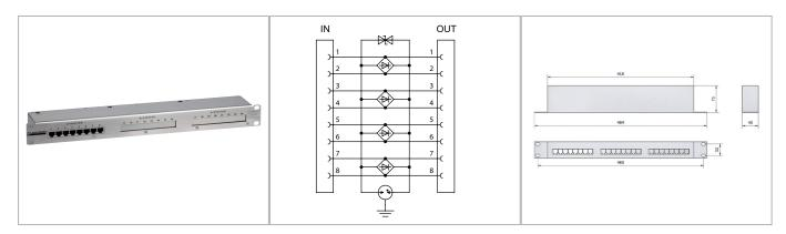
Compact surge protective module in 19" housing with only 1 HE (45 mm) for the protection of data networks and network devices such as hubs, switches, server and desktop computer. Easy installation and wiring in all 19" distribution and server racks possible. All 8 signal lines (4 pair of wires) are protected simultaneous
