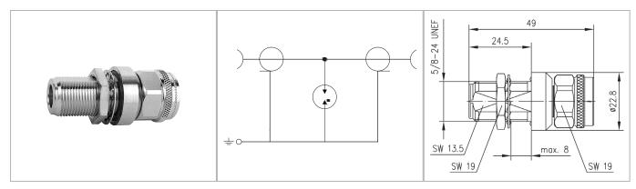
The devices are medium sized, precision, weatherproof connectors supplied with a screw coupling. Speciell design techniques for this series of connectors have resulted in excellent levels of performance with regard go return loss (VSWR) and intermodulation disortion.
