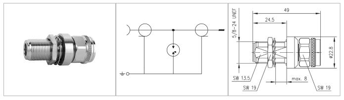
The devices are medium sized, precision, weatherproof connectors supplied with a screw coupling. Speciell design techniques for this series of connectors have resulted in excellent levels of performance with regard go return loss (VSWR) and intermodulation disortion. N surge supressor male (m)-female (f) with gas discharge arrester
