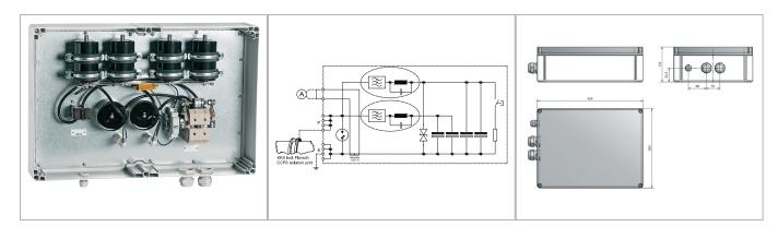
With an active cathodic corrosion protection the installation is permanently protected against the electrochemical process of corrosion. For that matter a grid supplied rectifier is inserted between the installation (e.g. a pipeline) and an anode that serves as earth electrode.
